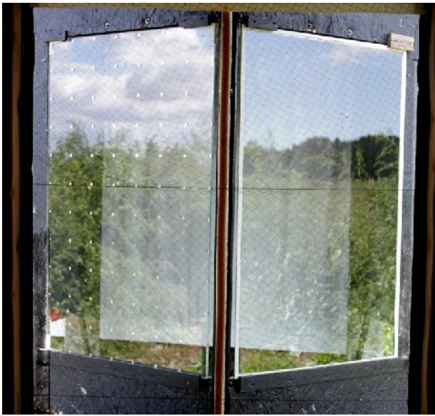
Figure 1: Test candidate “SEEN shiny” (left) and unmarked float glass reference (right) in the perspective of an approaching bird in the flight tunnel.
