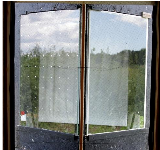
Figure 2: Test candidate “SEEN matt” to the left, float glass reference to the right.
