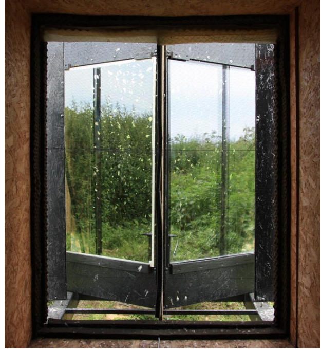
Figure 7: End of tunnel with pane holder and test pane. Left: float glass reference pane; right: Ornilux Mikado test pane. Vegetation and sky are reflected on both panes. The background of the panes can only be seen in the form of individual spots of light. The contrasts on the test pane (R.) are weaker than those on the reference pane (L.) The possible influence of different heights of vegetation is cancelled out by the continuous rotation of the tunnel and the equal frequency with which the test panes are positioned on the left and right side.
