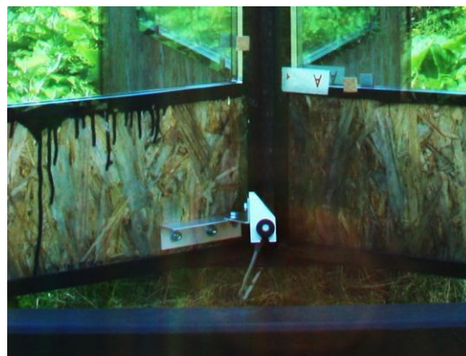
Figure 9: Photovoltaic sensor for measuring radiation behind the test panes.
