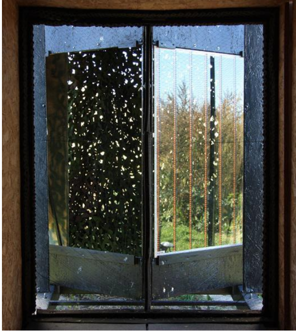
Figure 6: End of tunnel with pane holder and darkened area in the background of the panes. Left: no pane, unobstructed view of camouflage net (artificial background with light spots); right: black and orange reference test pane, reflection of vegetation outside right. The vertical black line is the reflection of the right screen, projected into the image from the right.
