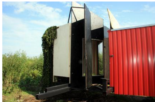
Fig. 5: Screens (black plates) restrict the birds' view to the extent of the glass panes. The side walls (white plate) and camouflage net (green curtain) reduce the light intensity in the background of the tunnel to \leq 25\text{W/m}^2 .
